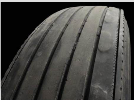
Depression Wear (Shoulder)
