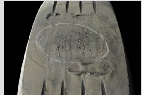
Brake Skid Damage
