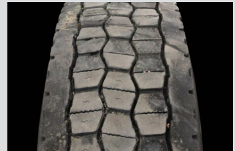
Cupping/Scallop/Alternate Lug Wear
