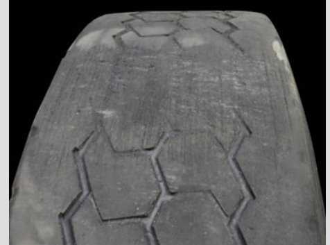
Brake Skid Damage
